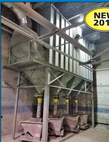
AGET Model FH585-4-SP Dusttop Filterkop Shaker-Type Dust Collector
